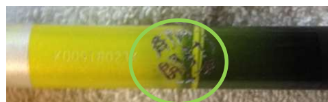
Appearance after the label has been peeled off the shaft
